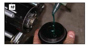
**11.** With the Turbo Lube cap filled with oil, position the cap perpendicular to the hub with the top thread of the cap lined up with the bottom thread of the threaded hub. Flip cap up 90 degrees and thread the cap onto the hub. If done correctly, no oil should spill from the cap. Torque cap to 10 ft/lbs.
