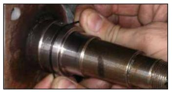
**4.** Once any and all burs and sharps have been removed, replace the old spindle/wear sleeve O-ring with a new O-ring; lightly lubricate the O-ring prior to assembly. Inspect O-ring for any damage prior to assembly over the spindle. Ensure O-ring is fully seated inside of the seal groove.
