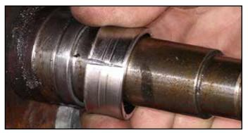
**2.** Once the press-fit bond of the wear sleeve has been broken, remove the old wear sleeve from the spindle
