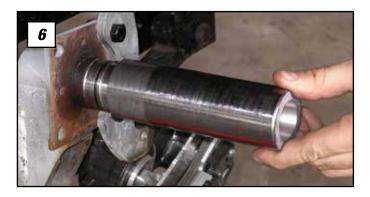
7. Once the wear sleeve is positioned with the wear sleeve assembly tool, strike the back of the assembly tool with a small sledge, or a large sized hammer. Make sure that the wear sleeve bottoms out on the on the spindle's wear sleeve machining detail.
