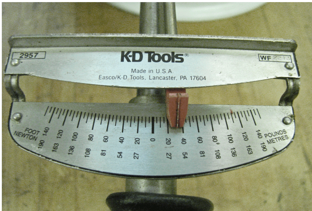
Photo 26 - For Reference, On this Traditional Beam Style Torque Wrench the Setting Reads 35 Foot Lbs, the Correct Torque Setting for the 2 Slider Pins.
