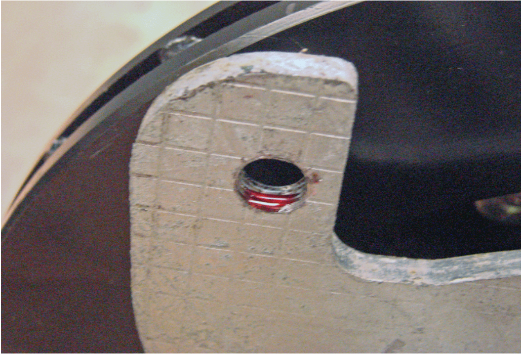
Photo 14 - A "Puddle" of the Liquid Red Thread Locker In the Bottom of the Threaded Hole, as Shown, Is All That's Required.
